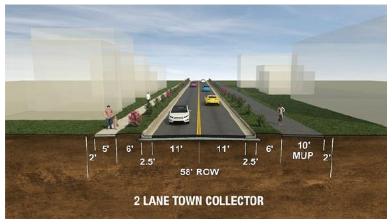
Cross Section 2- 2 Lane Town Collector Road
