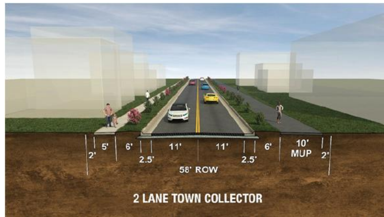
Cross Section 2- 2 Lane Town Collector Road
