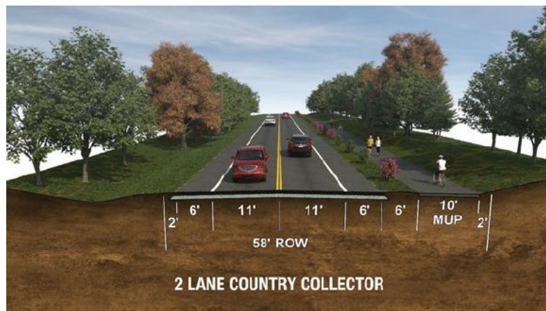
Cross Section 7- 2 Lane Country Collector Road
